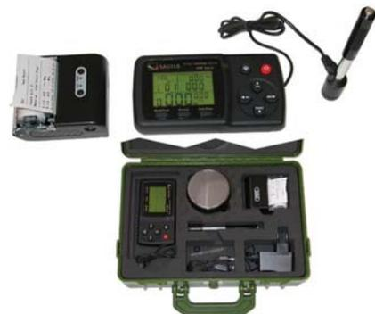
**DUROMETRI (hardness testers)**
